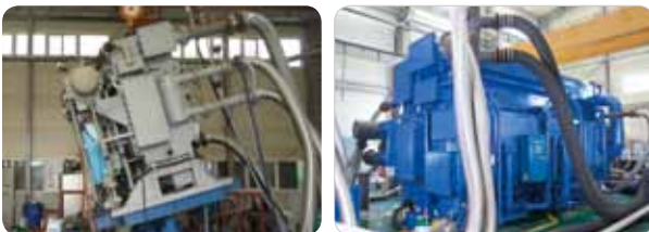
▲ High COP Single Effect 2-Lift Hot Water Driven Absorption Chiller
